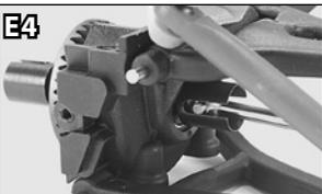
33. Slide the right-side bulkhead half onto the diff. Insert the right driveshaft into the diff cup and connect the two bulkhead halves together (E5). **Note:** When joining the two front bulkhead halves together, make sure to connect (key in) the steering bellcrank mount between the two halves (E6).
