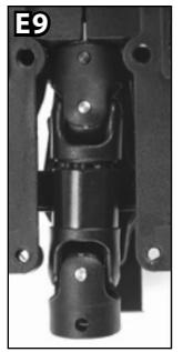
36. Slide the front end assembly onto the chassis in the same manner it was removed. Make sure to reconnect the front center driveshaft to the front output shaft of the transmission. Secure it with the same screw pin (E10). Next, secure the front end to the chassis with the same two 3x10mm button head screws (E11).
